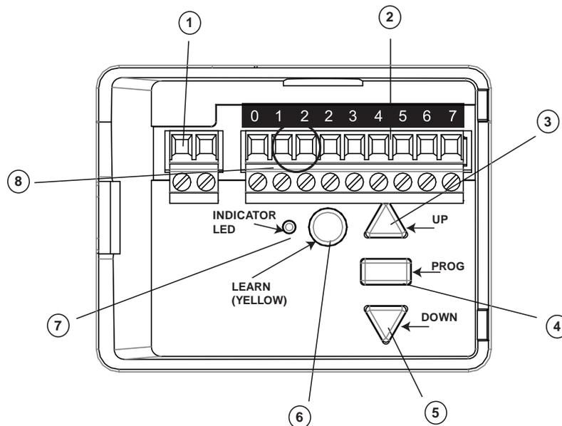
**NOTE: Door in Door Connections 4 & 5** (used where built-in pedestrian doors are installed within a garage door).
